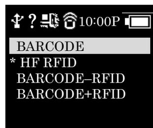
**"BARCODE "**: Set up the exclusive barcode mode and, read the only barcode when user pushes the scan button
