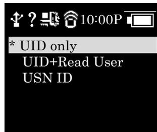
**"UID only"**: Output the UID (Unique Identification Number) of HF RFID Tag
